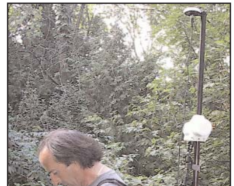
GSM-19 with internal GPS board. Small antenna attaches above sensor.
