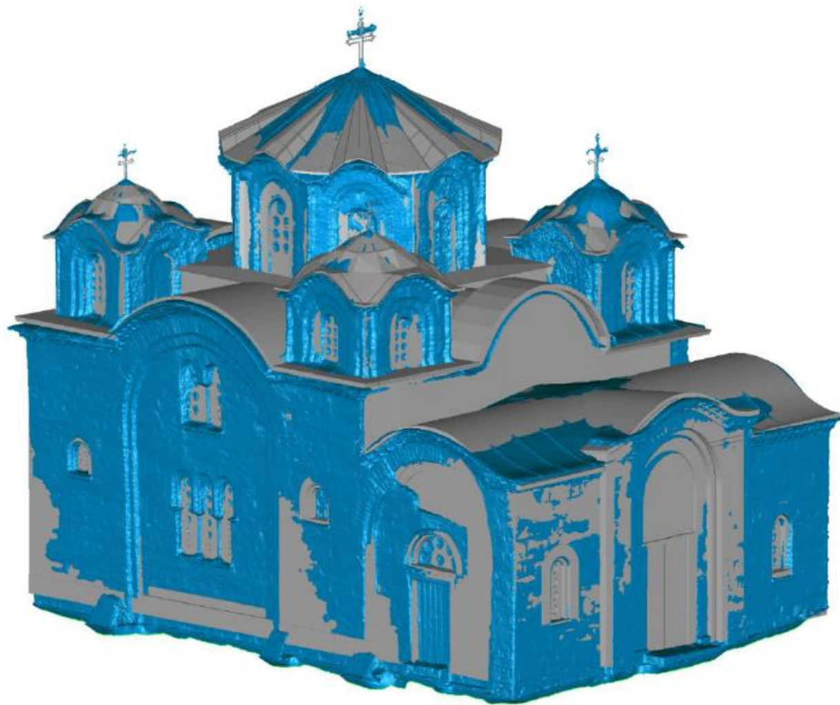
Comparison of both 3D models: BIM geometrical basic model (grey), photogrammetrical model (blue)
